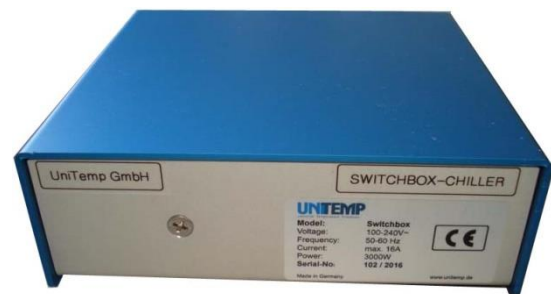
Figure 4: Front side of external switchbox
